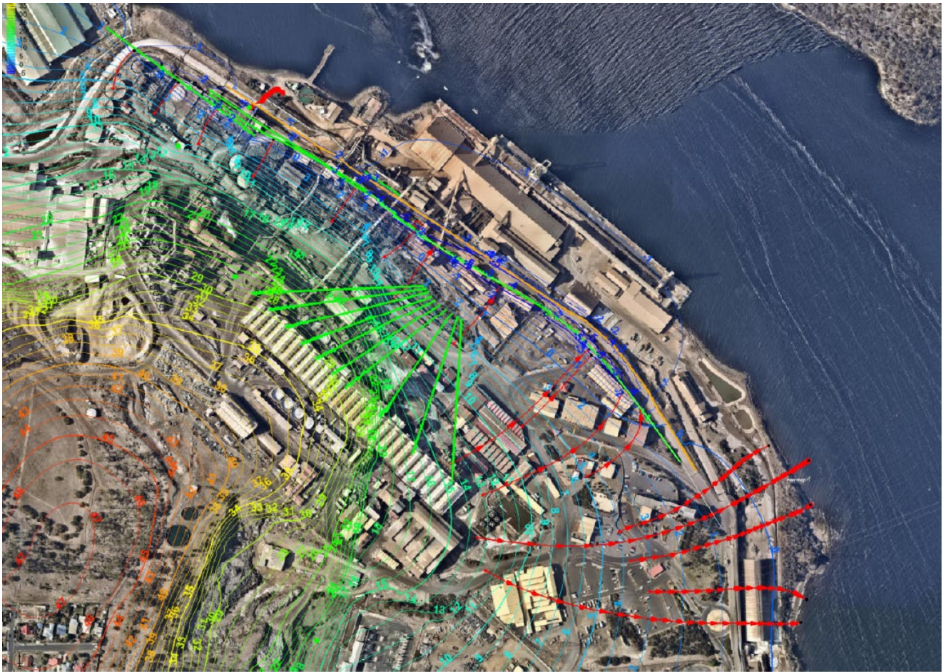
Figure 4-51 Modelled groundwater flow for the central and southern section of the site with the new grout curtain and horizontal drain in place
