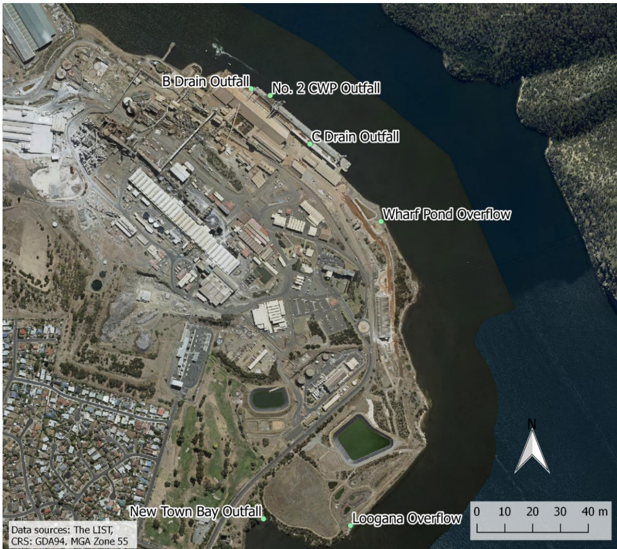
Figure 4-16 Surface water discharge monitoring locations – all points are emergency stormwater overflow points
