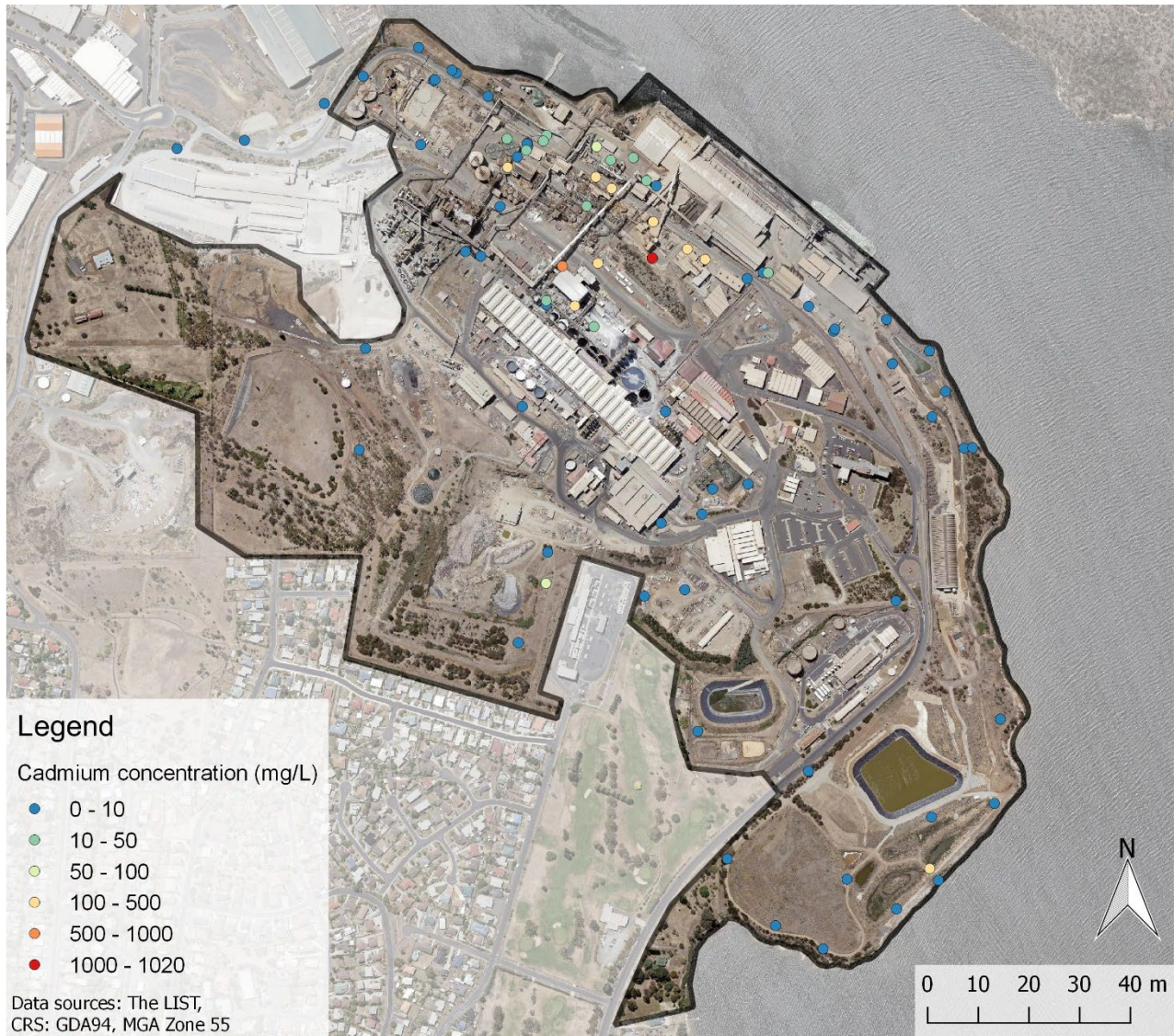
Figure 4-30 Cadmium (mg/L) in groundwater beneath the NH site from 2021 groundwater monitoring data
