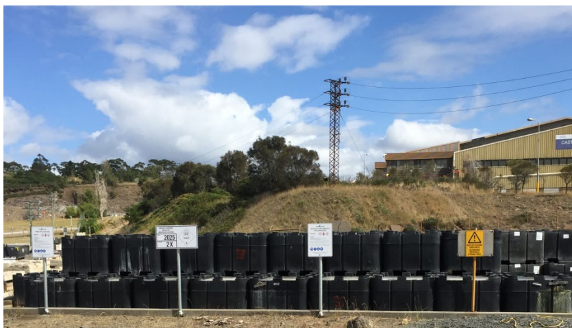
Figure 4-85 Purpose built containers containing Mercury Filter Cake, pre-treatment
