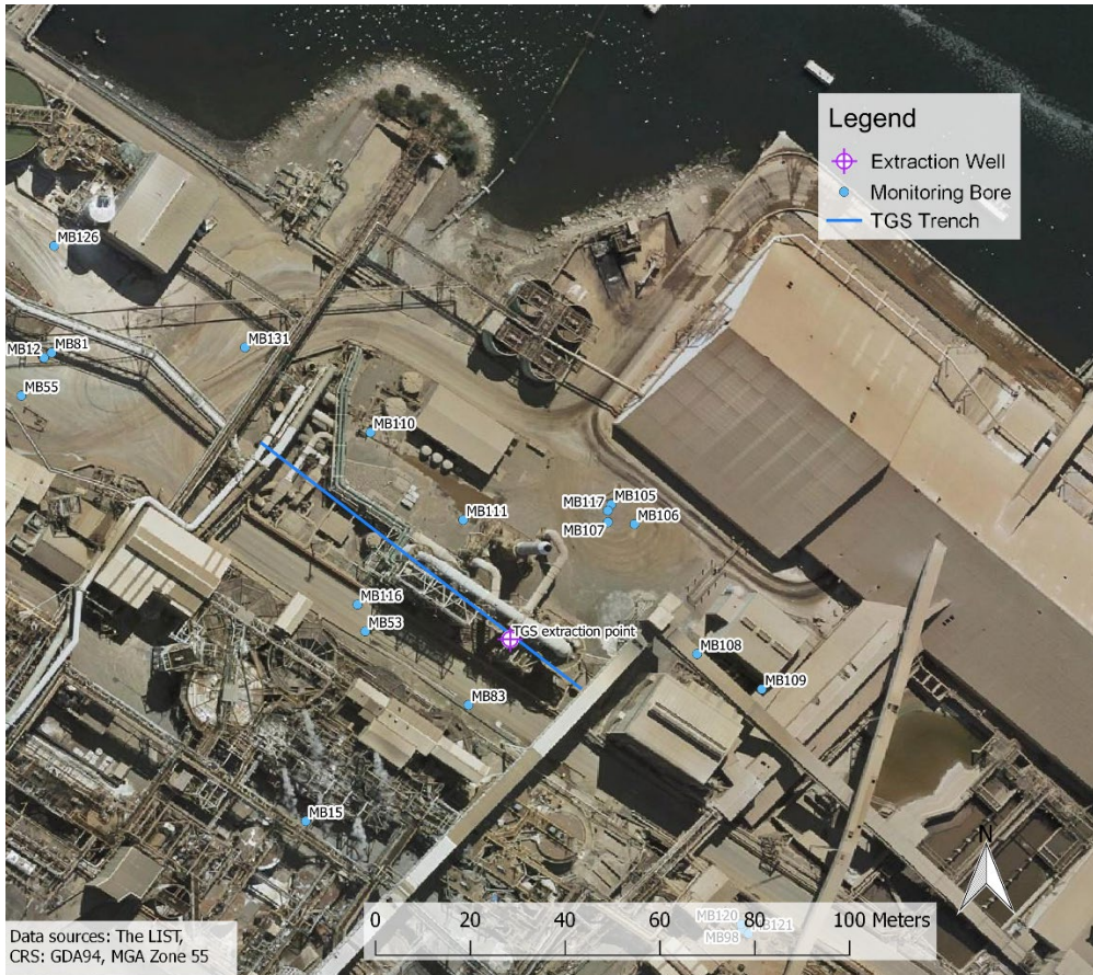
Figure 4-42 Location of Tail Gas Scrubber Trench Extraction System
