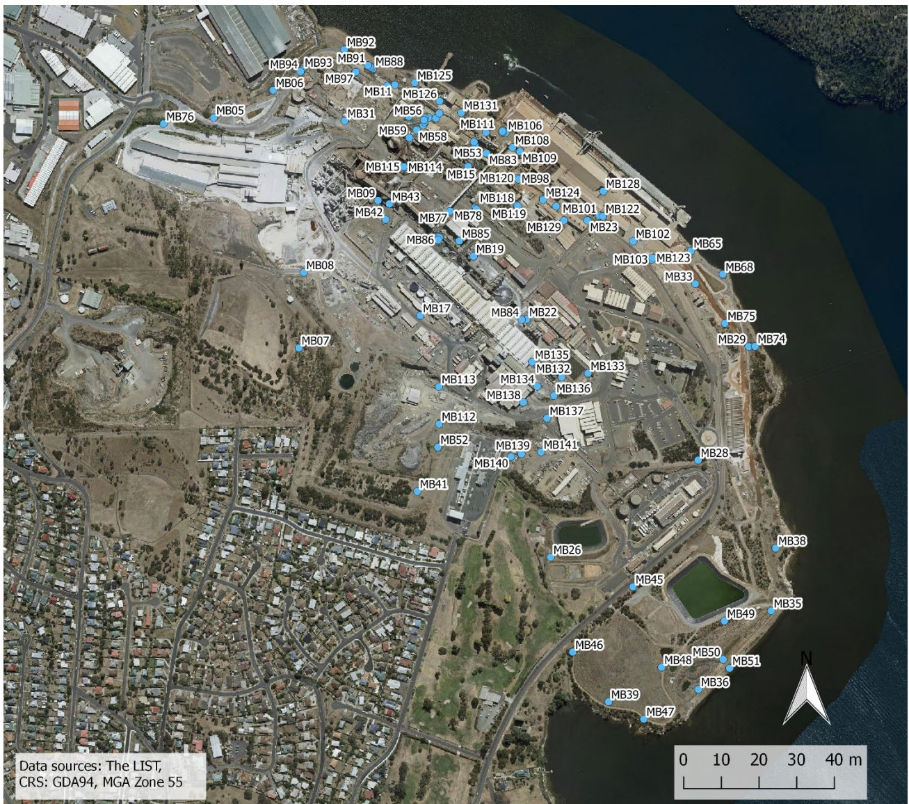
Figure 4-17 Groundwater monitoring borehole locations
