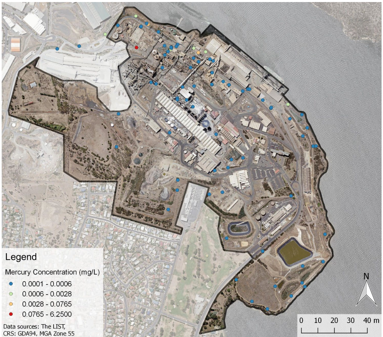
Figure 4-31 Mercury (mg/L) in groundwater beneath the NH site from 2021 groundwater monitoring data
