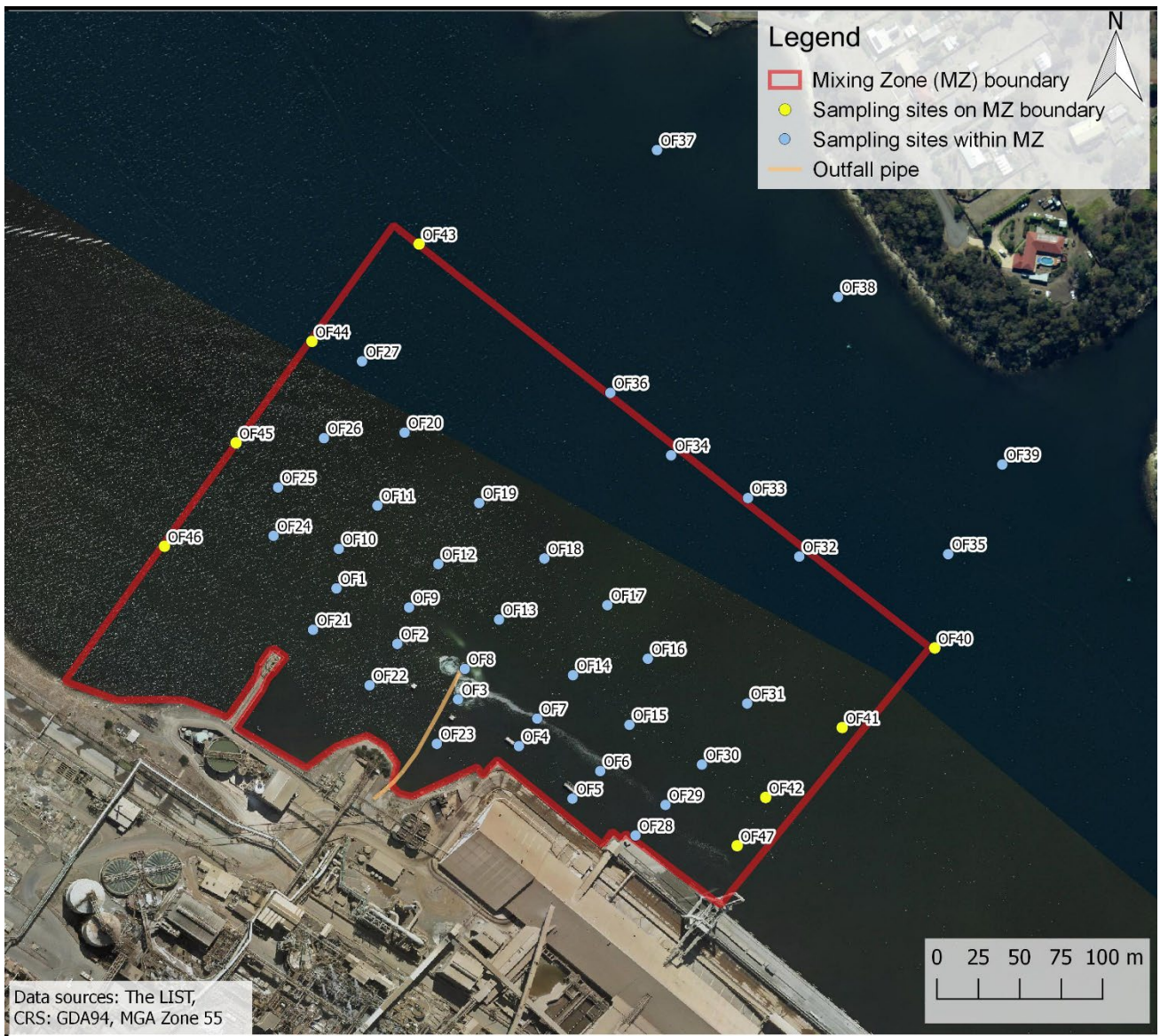
Figure 4-52 Point source mixing zone boundary
